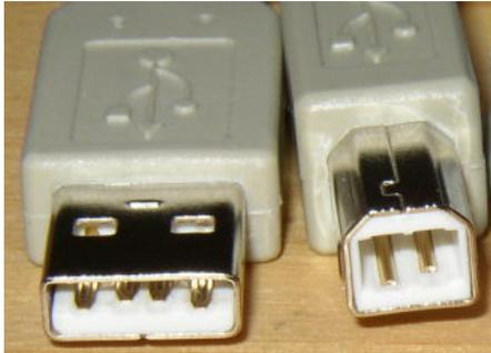
Usually a PC / notebook provides type A socket (rectangular connector, see left side of picture). The DALI controller USB input is type B (square connector, see right side of picture).
